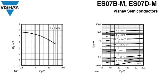
Figure 3. Typ. Diode Capacitance vs. Reverse Voltage
