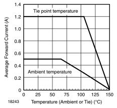
Figure 2. Forward Current Derating Curve
