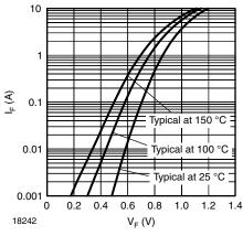
Figure 1. Typical Forward Characteristics
