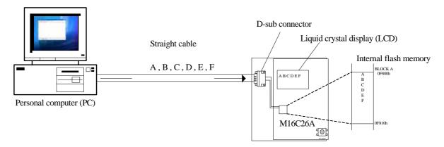
When SW1 is depressed, the data displayed on LCD is saved in the internal flash memory.
