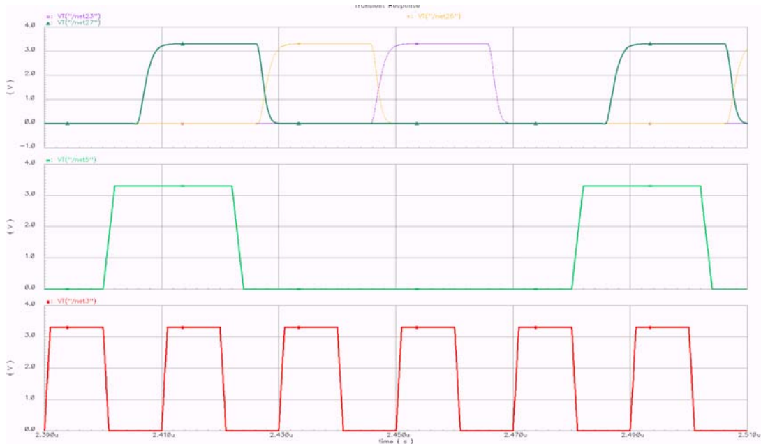
Figure 16: X-addressing. From bottom to top: Clock_x, Sync_x, internal selection pixel 1&2, internal selection pixel 3&4, internal selection pixel 5 & 6.
