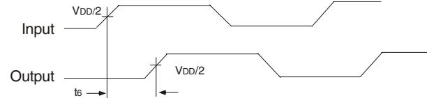
*Input to Output Propagation Delay*
