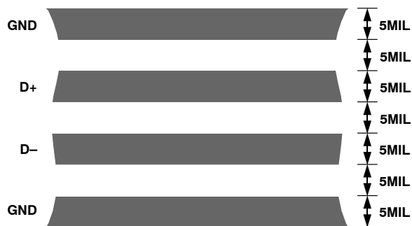
Figure 34. Typical Arrangement of Signal Tracks
