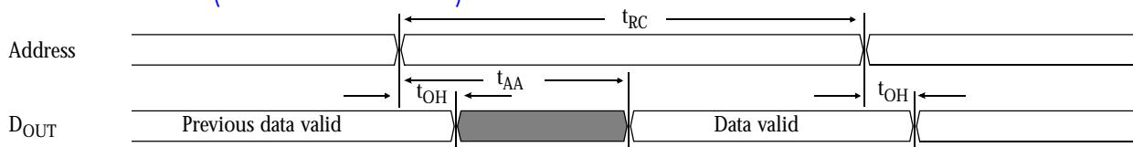
Read waveform 2 (Chip enables,  $\overline{OE}$ ,  $\overline{UB}$ ,  $\overline{LB}$  controlled)<sup>3,6,8,9</sup>
