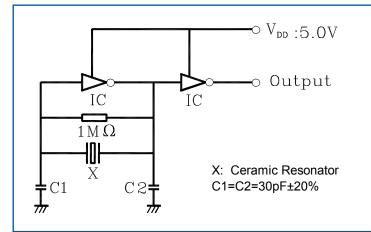
Parts shall be measured under a condition (Temp.:  $20\pm15^{\circ}$ C, Humidity:  $65\pm20\%$  R.H.) unless the standard condition (Temp:  $25\pm2^{\circ}$ C, Humidity:  $65\pm5\%$  R.H.) is regulated to measure
