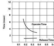
Coil Power (W) Test relay: OJE-SH-112LMH
