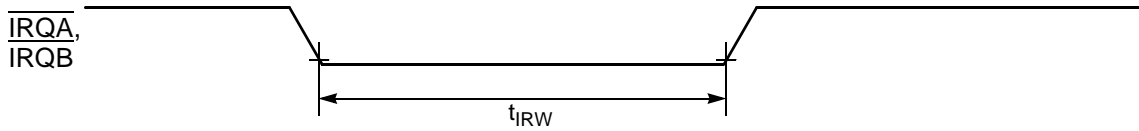
Figure 10-6 External Interrupt Timing (Negative-Edge-Sensitive)
