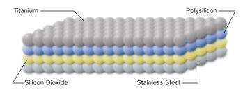
The thin film is atomically fused directly to the steel surface of the gauge beam and therefore follows the shape of the beam very accurately. This atomic fusion is the foundation for excellent performance and stability.
