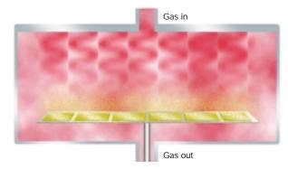
Stainless steel Psibar wafers lie in a gas stream of plasma-enhanced gases. The PECVD process is used because it deposits high quality silicon at low temperature, which does not affect the state of the steel gauge. After deposition, the silicon is ion implanted to modify resistivity.
