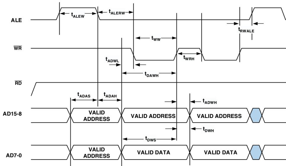
NOTE: MEMORY WRITES ALWAYS OCCUR IN GROUPS OF FOUR BETWEEN ALE CYCLES. THIS FIGURE ONLY SHOWS TWO MEMORY WRITES IN ORDER TO PROVIDE THE NECESSARY TIMING INFORMATION.
