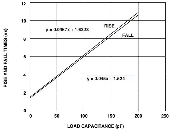
Figure 31. Typical Output Rise/Fall Time (20% to 80%, V<sub>DDEXT</sub> = Max)
