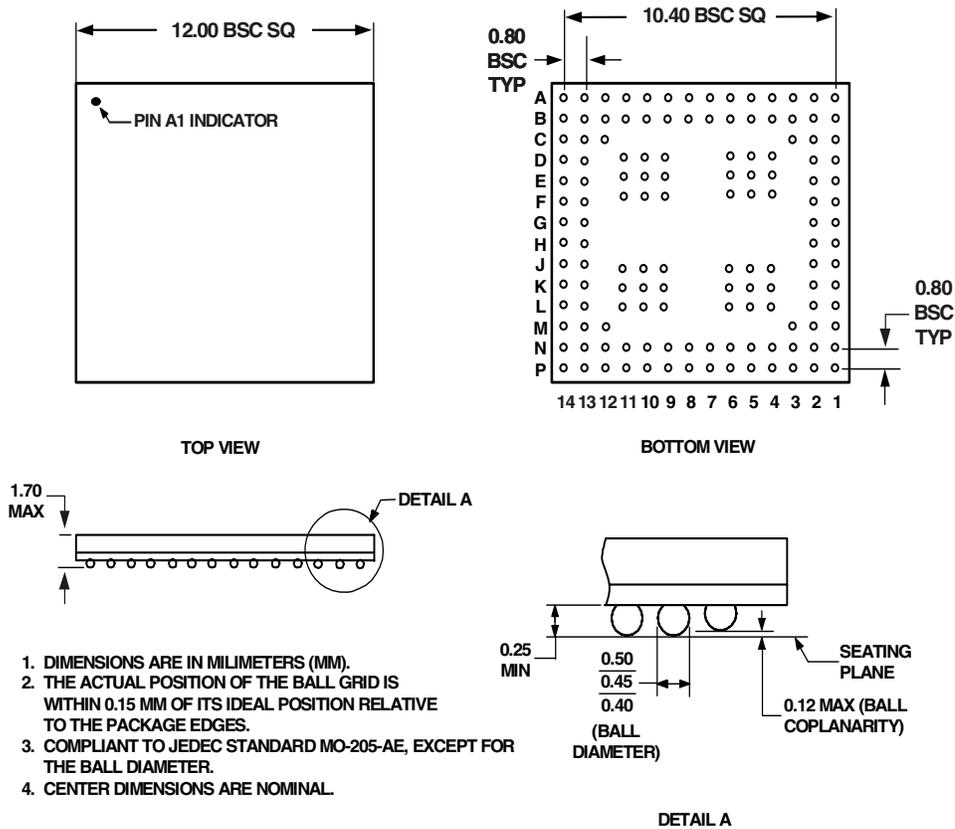
Figure 36. 136-Lead Chip Scale Package Ball Grid Array [CSP\_BGA](BC-136-2)
