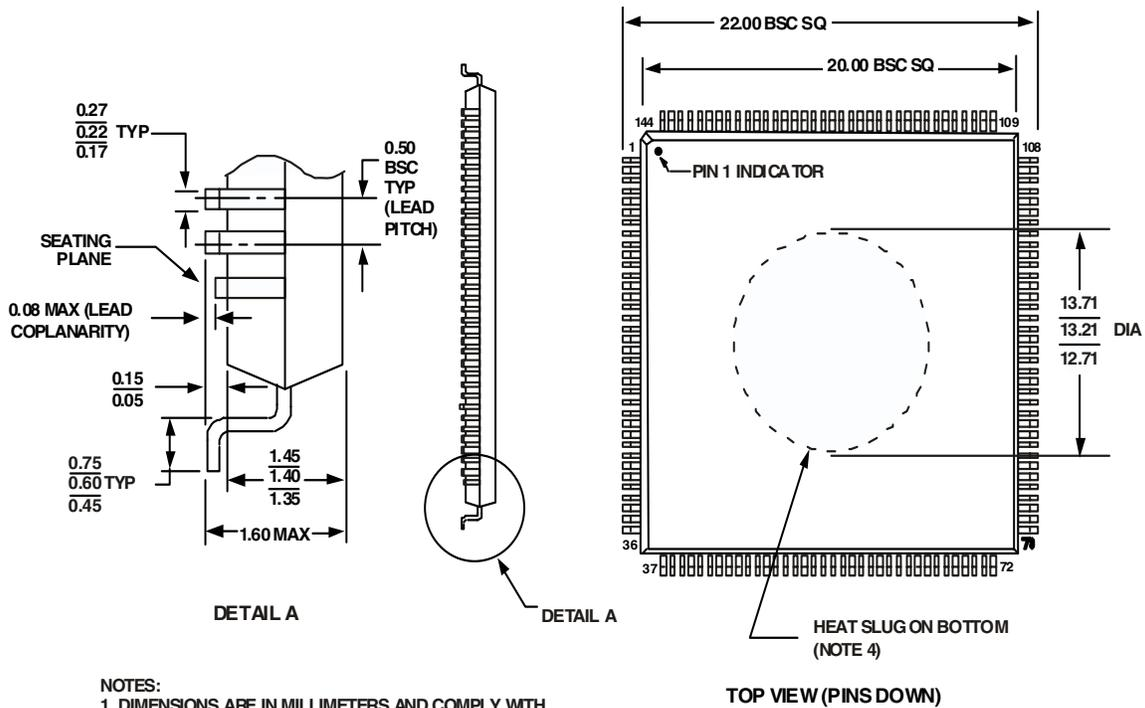
Figure 35. 144-Lead Low Profile Quad Flat Package, with Integrated Heatsink [LQFP\_INT\_HS] (SQ-144-3)
