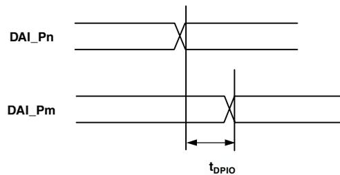
Figure 14. DAI Pin to Pin Direct Routing
