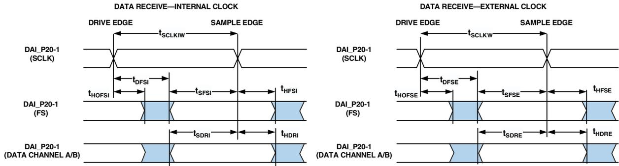
NOTE: EITHER THE RISING EDGE OR FALLING EDGE OF SCLK (EXTERNAL), SCLK (INTERNAL) CAN BE USED AS THE ACTIVE SAMPLING EDGE.
