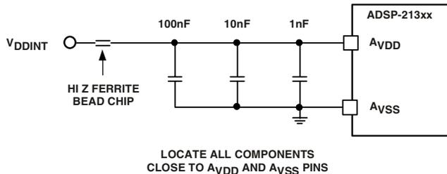
Figure 4. Analog Power ( $A_{VDD}$ ) Filter Circuit
