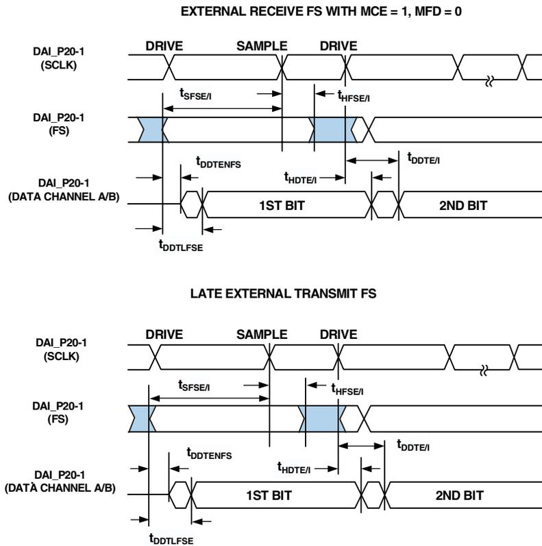
NOTE: SERIAL PORT SIGNALS (SCLK, FS, DATA CHANNEL A/B) ARE ROUTED TO THE DAI\_P20-1 PINS USING THE SRU. THE TIMING SPECIFICATIONS PROVIDED HERE ARE VALID AT THE DAI\_P20-1 PINS.
