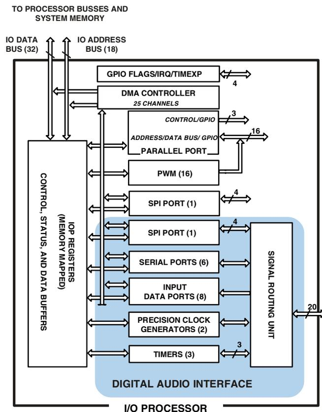
Figure 3. ADSP-21363 I/O Processor and Peripherals Block Diagram
