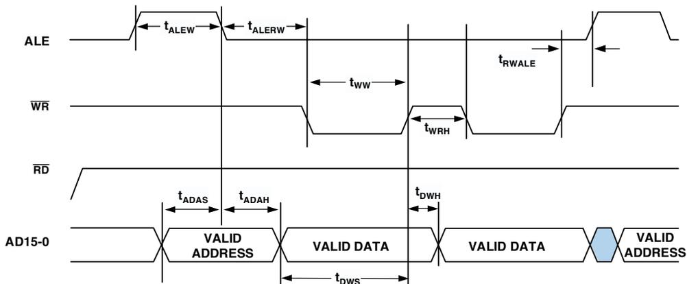
NOTE: FOR 16-BIT MEMORY WRITES, WHEN EMPP = 0, ONLY ONE  $\overline{WR}$  PULSE OCCURS BETWEEN ALE CYCLES. WHEN EMPP = 0, MULTIPLE  $\overline{WR}$  PULSES OCCUR BETWEEN ALE CYCLES. FOR COMPLETE INFORMATION, SEE THE ADSP-2136X SHARC PROCESSOR HARDWARE REFERENCE.
