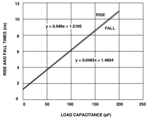
Figure 32. Typical Output Rise/Fall Time (20% to 80%, V<sub>DDEXT</sub> = Min)
