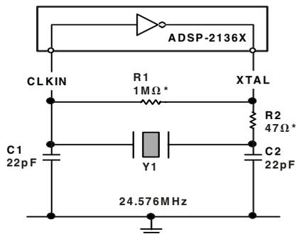
R2 SHOULD BE CHOSEN TO LIMIT CRYSTAL DRIVE POWER. REFER TO CRYSTAL MANUFACTURER'S SPECIFICATIONS
