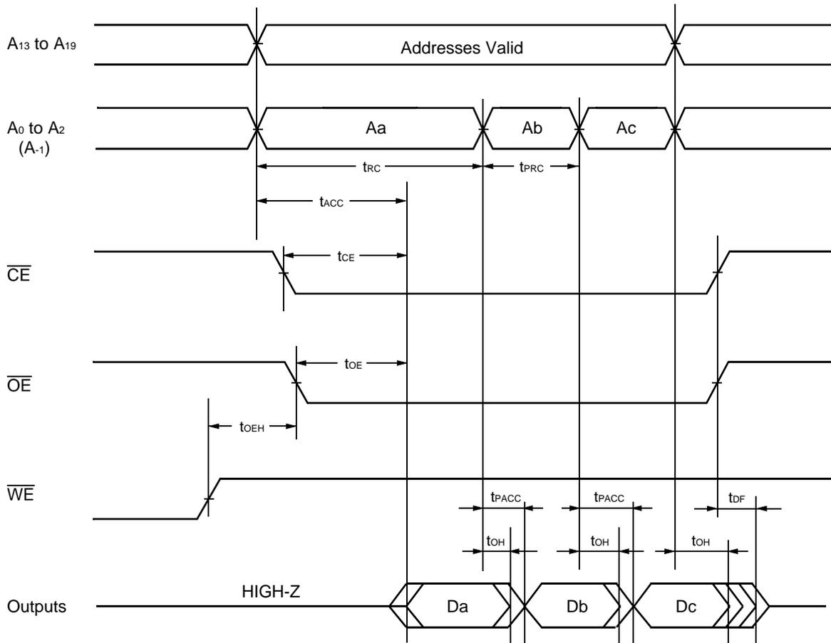
**Figure 5.2 AC Waveforms for Page Read Mode Operations**
