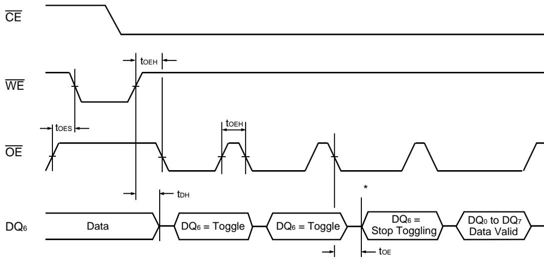
\* :  $DQ_6$  = Stops toggling. (The device has completed the Embedded operation.)
