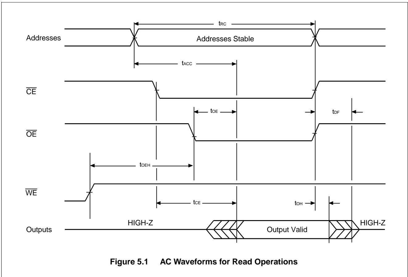
Figure 5.1 AC Waveforms for Read Operations
