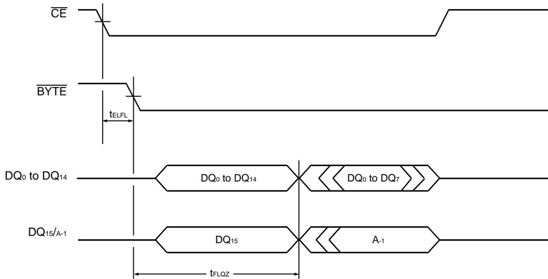
**Figure 12** Timing Diagram for Byte Mode Configuration
