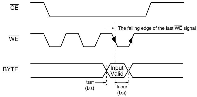
Figure 13  $\overline{BYTE}$  Timing Diagram for Write Operations
