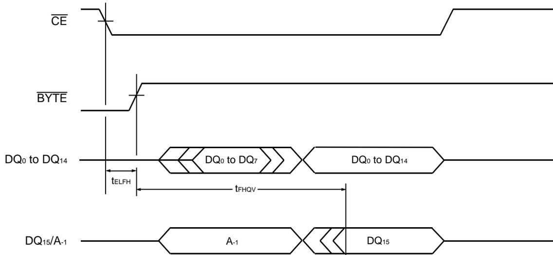
**Figure 11** Timing Diagram for Word Mode Configuration
