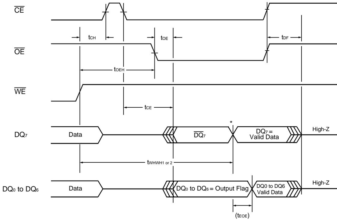
\* :  $DQ_7$  = Valid Data (The device has completed the Embedded operation.)
