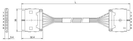
NOTE: Diagram numbers 1 through 6 indicate contact numbers. Note that indications do not appear on the connectors.
