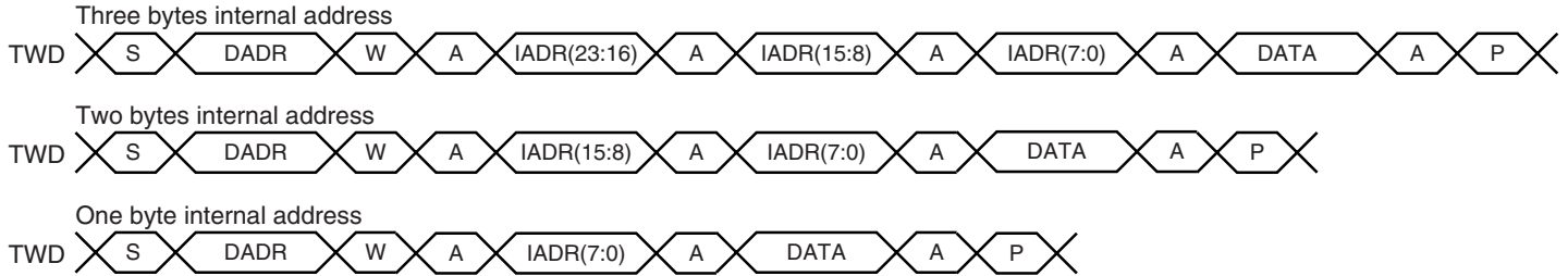
Figure 21-5. Master Write with One, Two or Three Bytes Internal Address and One Data Byte
