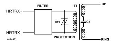
Figure 13. HOME PHONE NETWORKING ISOLATION/FILTER/PROTECTION CIRCUIT
