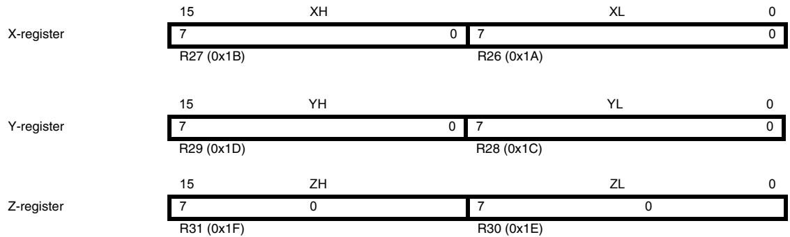
Figure 6-3. The X-, Y-, and Z-registers
