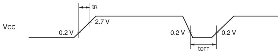
Note : Extreme variations in power supply voltage may activate a power-on reset. As the illustration below shows, when varying power supply voltage during operation, the use of a smooth voltage rise with suppressed fluctuation is recommended. Also in this situation, the PLL clock on the device should not be used, however it is permissible to use the PLL clock during a voltage drop of 1V/s or less.
