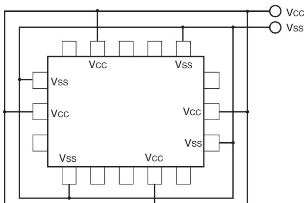
Power supply input pins (V<sub>CC</sub>/V<sub>SS</sub>)
