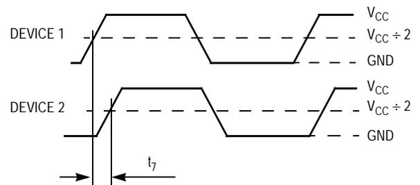
Figure 4. Device-to-Device Skew
