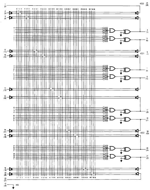
Note. Numbers in parentheses refer to the PLCC pin number, PLCC pins 1, 8, 15, and 22 are not connected.
