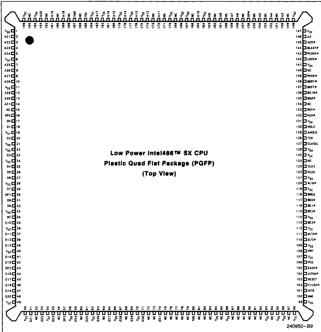
Figure 16-3. Low Power Intel486™ SX CPU 196-Lead PQFP Pinout
