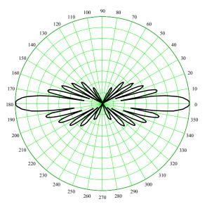
**Elevation Pattern** Polar Plot Center = -40dB 5 dB / radial division 10 degree / angular division
