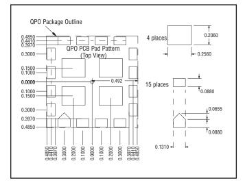
Figure 14 - LAND GRID ARRAY PCB Solder Mask Openings (dimensions in inches)
