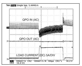
*Figure 2* – *Typical performance with a 3.3 Volt converter, showing 1 to 10 A load step.*
