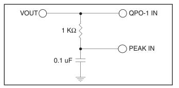
Figure 5 – Peak detect disable circuit.
