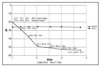
Figure 10 - Attenuation vs. power dissipation with slope adjust.
