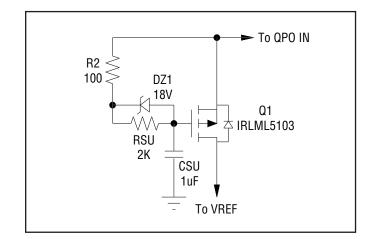
Figure 11 - Zero Headroom Start-up Circuit.
