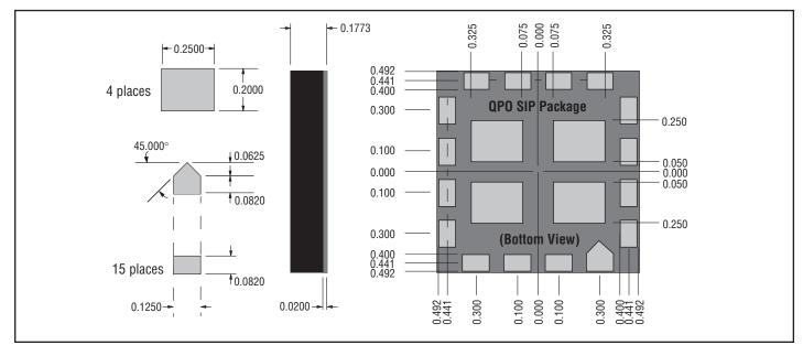
Figure 13 - Package dimension drawing (dimensions in inches)
