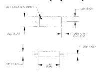
$\begin{array}{ll} \pm .002 \\ \text{Leads are .012 (.31) diameter (std.).} & \text{Dimensions in (i)'s are mm. Tolerance: } .000 \pm .010 \\ & \pm .010 \\ & \pm .002 \\ \text{May be supplied as tabs: .025 (.64) Wide, .006 (.15) Thick (opt.).} \end{array}$
