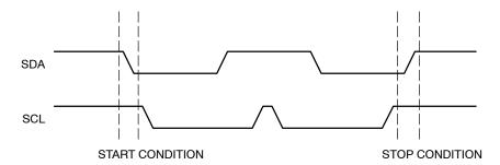
Figure 4. Start/Stop Timing
