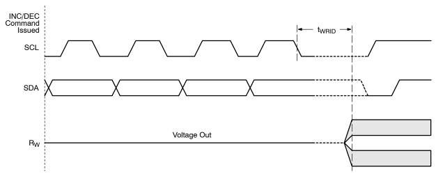
Figure 13. Increment/Decrement Timing Limits
