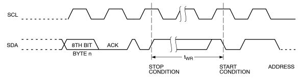
Figure 3. Write Cycle Timing
