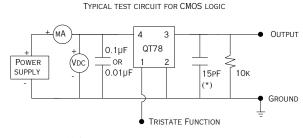
(\*) CL includes probe and JIG capacitance
