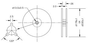
Dimensions are in mm. Tape is compliant to EIA-481-A.
