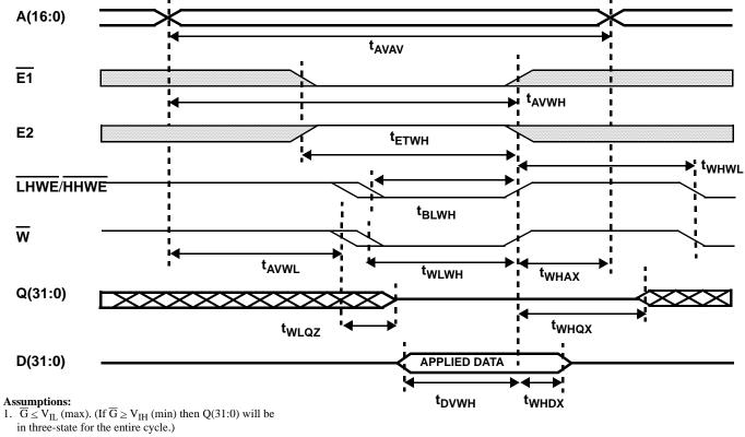
Figure 4a. SRAM Write Cycle 1:  $\overline{W}$  - Controlled Access
