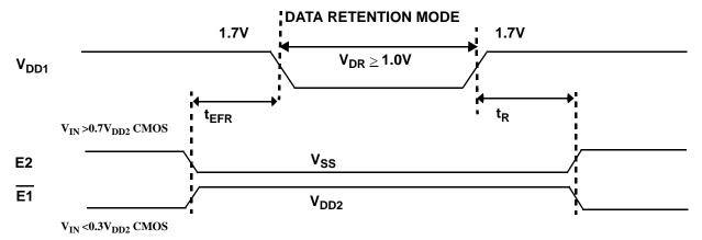
Figure 5. Low V<sub>DD</sub> Data Retention Waveform
