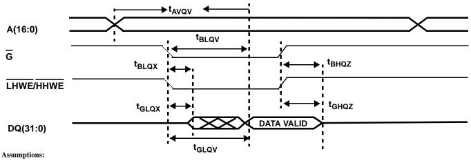
1.  $\overline{E1} \leq V_{IL} \ (\text{max})$  , E2 and  $\overline{W} \geq V_{IH} \ (\text{min})$
