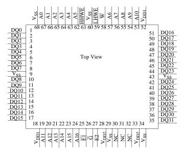
Figure 2. 15ns SRAM Pinout (68)
