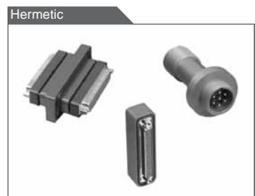
**FEATURES:** Intended for use as an electrical feedthrough in high vacuum applications • Leakage rate:  $5 \times 10^{-9}$  mbar.l/s @ vacuum  $1.5 \times 10^{-5}$  atm • Signal, power, coax and high voltage versions available • Connectors can be mounted on flange assembly per customer specification
