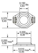
\* Allow an additional 0.01/0,254 in length and 0.005/0,127 in height for optional tin-lead and tin-silver-copper application.
