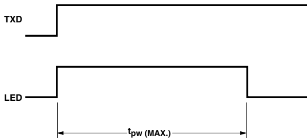
Figure 9. TXD "Stuck ON" protection.
