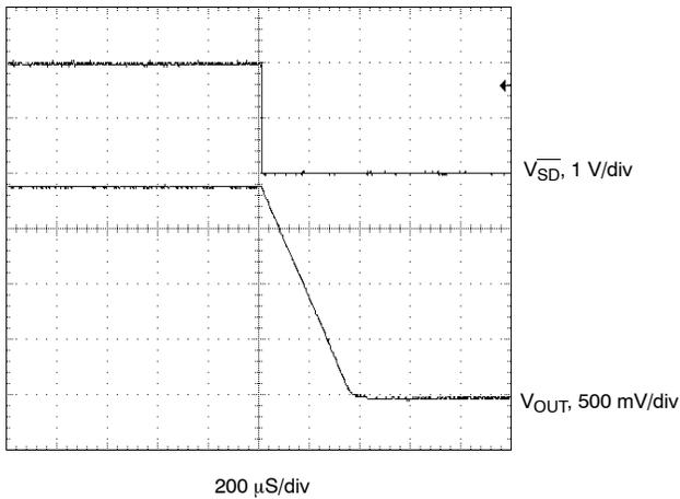
Enable Switching,  $R_{LOAD} = 4\ \Omega$
