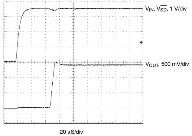
Shutdown,  $R_{LOAD} = 4\ \Omega$
