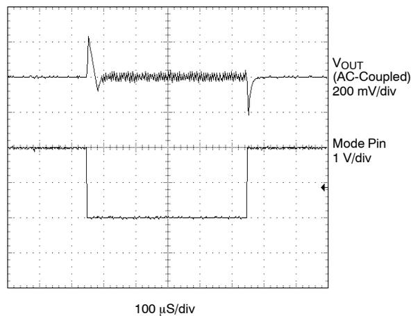
**TYPICAL LOAD TRANSIENT WAVEFORMS ( $V_{IN} = 3.6\text{ V}$ ,  $V_{OUT} = 1.9\text{ V}$ )**
