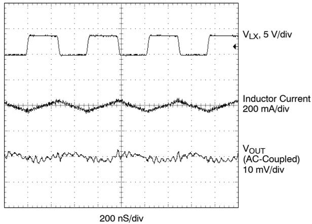
PSM Mode Light-Load Switching Waveforms,
