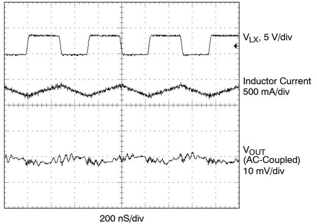
PWM Mode Light-Load Switching Waveforms,
