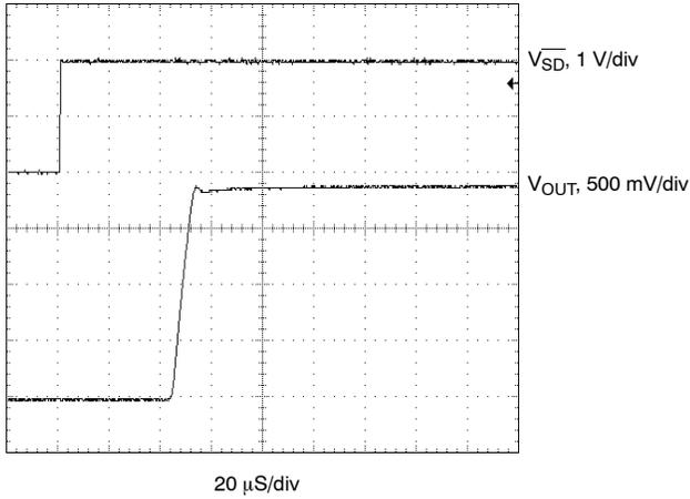
Start-Up,  $V_{IN} = V_{SD} = 3.6\text{ V}$ ,  $R_{LOAD} = 4\ \Omega$
