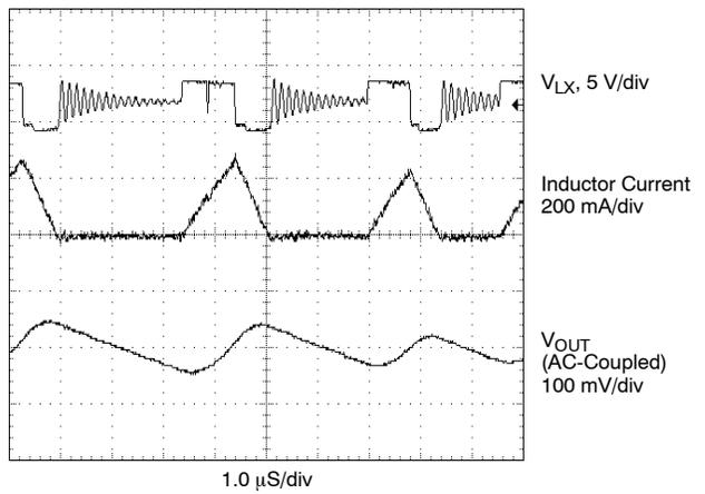
PSM Mode Light-Load Switching Waveforms,
