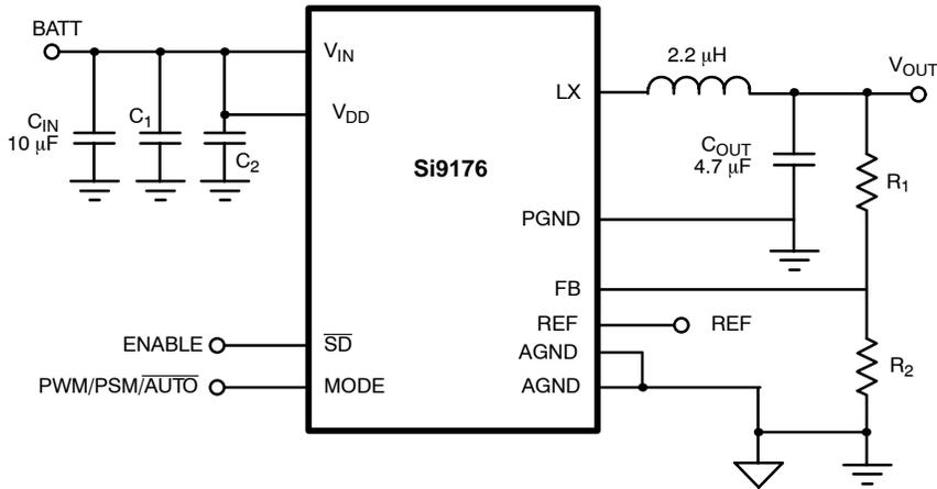
$C_{IN} = 10 \mu\text{F}$ , Ceramic, Murata GRM42-2X5R106K16
