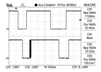
Figure 2. Actual Rotary Encoder waveform
