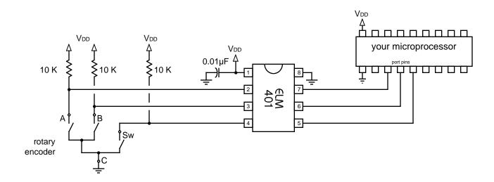
Figure 4. Connecting the ELM401 to a microprocessor
