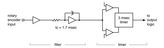
Figure 3. Internal Debouncing Logic
