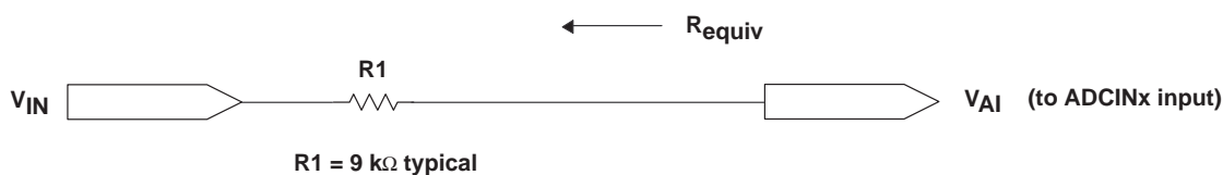
Figure 47. Typical ADC Input Pin Circuit
