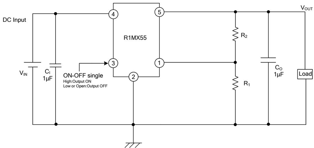
■ ELECTRICAL CHARACTERISTICS MEASURING CIRCUIT(FOR SOT-89-5)
