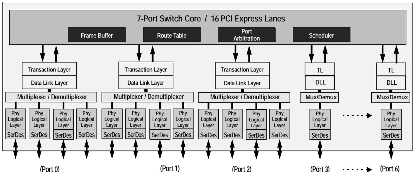
Figure 1 Internal Block Diagram
