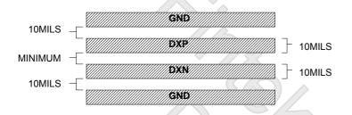
Use wide tracks to minimize inductance and reduce noise pickup. 10 mil track minimum width and spacing is recommended.
