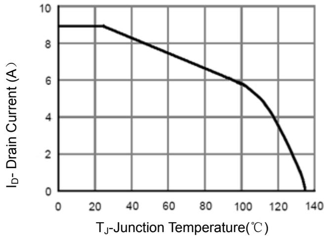
**Figure 4 Drain Current**
