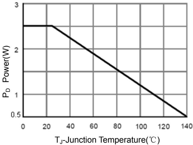
**Figure 3 Power Dissipation**
