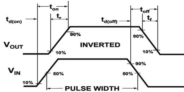
**Figure 2: Switching Waveforms**
