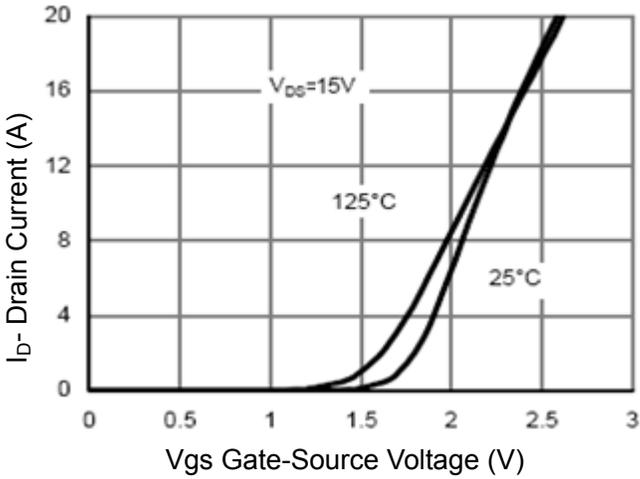
**Figure 7 Transfer Characteristics**
