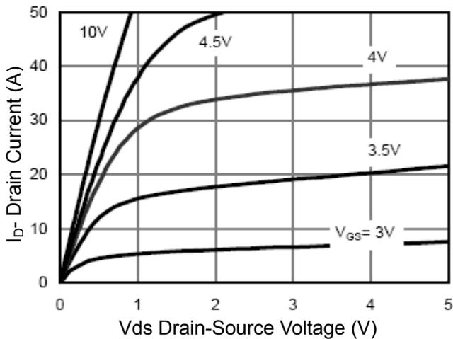
**Figure 5 Output CHARACTERISTICS**
