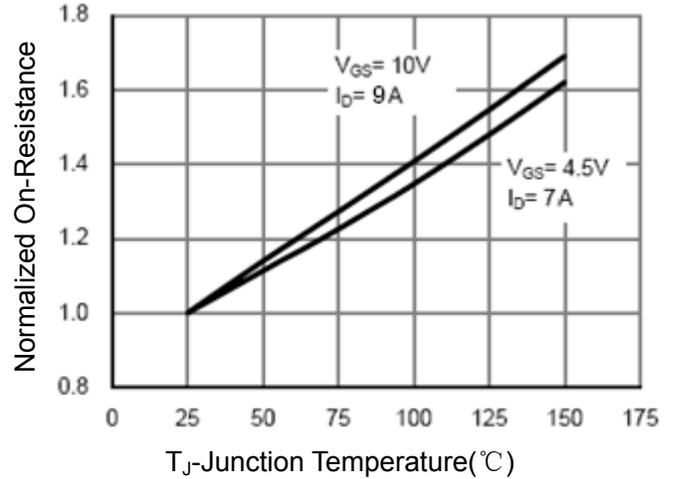
**Figure 8 Drain-Source On-Resistance**
