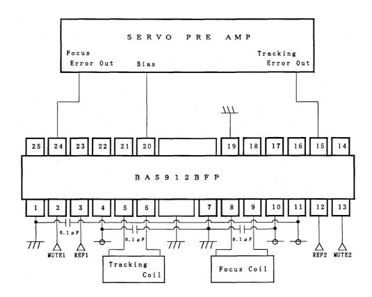
When used at Pre Vcc > Pow Vcc + VF and in the standby mode, REF1 (PIN3) and REF2 (PIN12) must be set to open, or 0.5V or less. When used with REF1 (PIN3) and REF2 (PIN12) shorted; or MUTE1 (PIN2) and MUTE2 (PIN13) shorted, each microcomputer output must be able to supply a current of 300μA or so.
