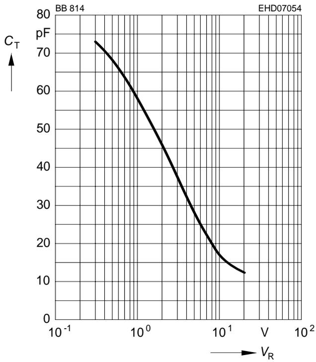
**Capacitance ratio  $C_{Tref}/C_T = f(V_R)$**
