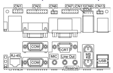
• CN1: Internal LAN Connector (5x2 Header)
