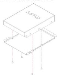
2. Place the whole HDD set on the chassis.
