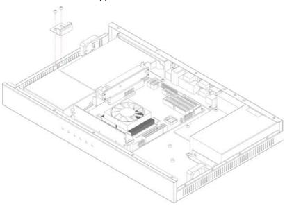
5. Completed assembly of HDD & PCI card as the following picture.
