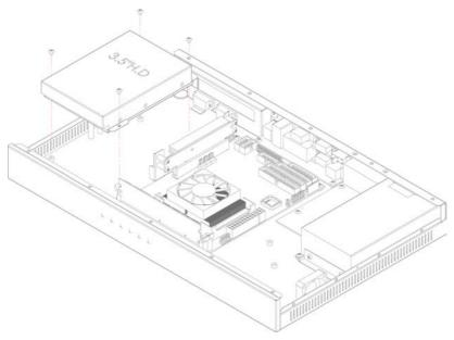
3. Insert PCI card to PCI extension slot, and fix it with a screw.
