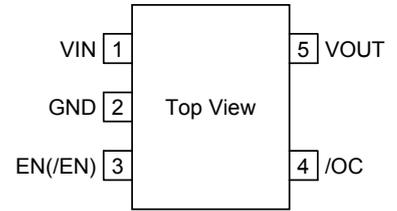
Fig.40 Pin configuration
