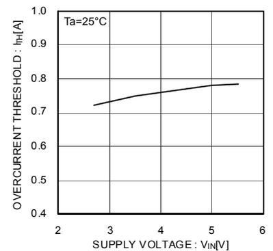
Fig.12 Over-current threshold
