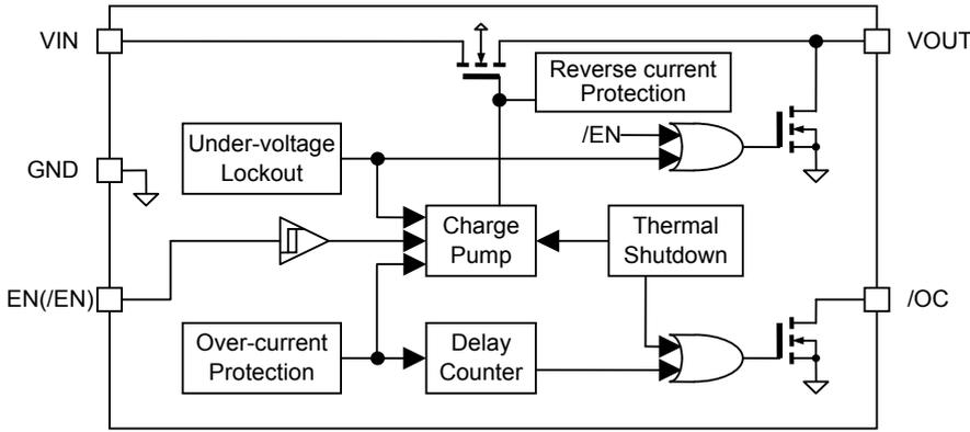
Fig.39 Block diagram
