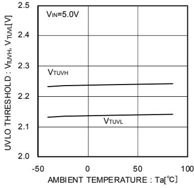
Fig.16 UVLO threshold
