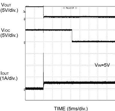
Fig.36 Over-current response 1Ω load to enabled device
