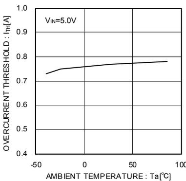
Fig.13 Over-current threshold
