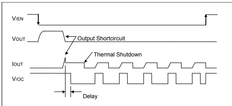
Fig.43 Over-current detection, Thermal shutdown timing (BD2247G)
