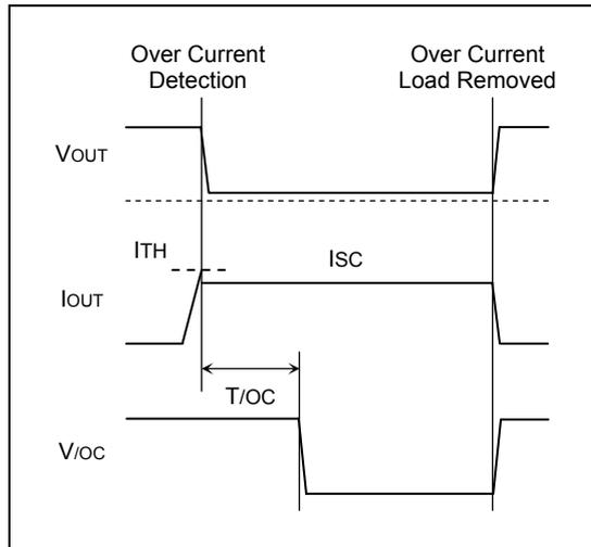
Fig.41 Over-current detection
