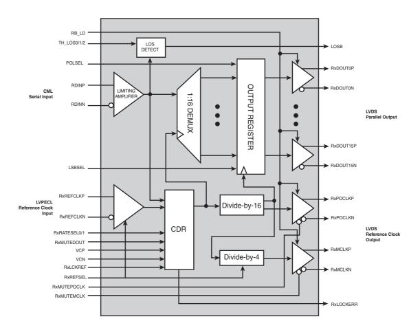
The BCM8125 is a fully integrated MSA-compatible quad-rate SONET/SDH/10GE receiver operating at OC-192/STM-64, 10GE, and two different FEC (Forward Error Correction) data rates (9.953, 10.3125, 10.664, and 10.709 Gbps) with deserializer, clock and data recovery (CDR), and loss-of-signal (LOS) detection circuitry. The BCM8125 provides high-jitter tolerance and low-jitter generation to comply with Optical Internetworking Forum (OIF), IEEE 802.3ae, Telcordia, ANSI, and ITU-T standards.
