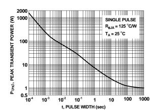
Figure 12. Single Pulse Maximum Power Dissipation
