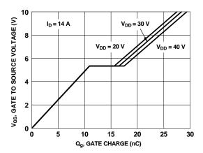
Figure 7. Gate Charge Characteristics
