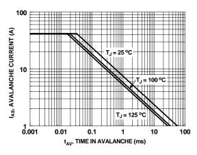
Figure 9. Unclamped Inductive Switching Capability
