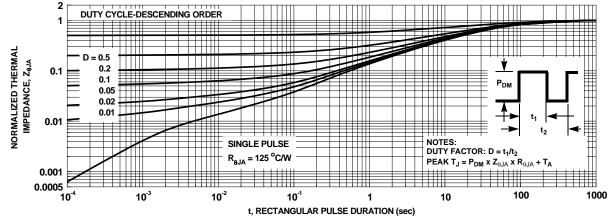
Figure 13. Junction-to-Ambient Transient Thermal Response Curve
