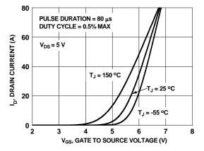
Figure 5. Transfer Characteristics
