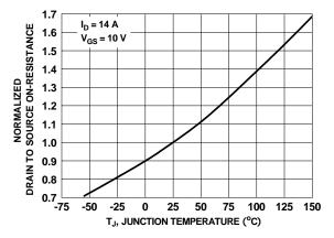
Figure 3. Normalized On-Resistance vs Junction Temperature
