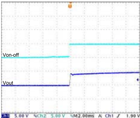
Graph 9: Using ON/OFF Voltage Start-Up and Vo Rise Characteristic (Nominal Vin and Full Load)
