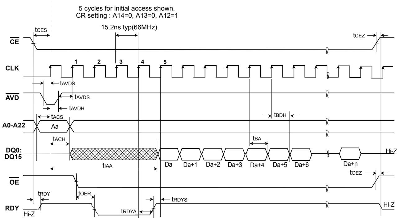
Figure 4: Continuous Burst Mode Read (66MHz)
