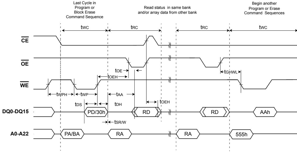
**Figure 17: Read While Write Operation**
