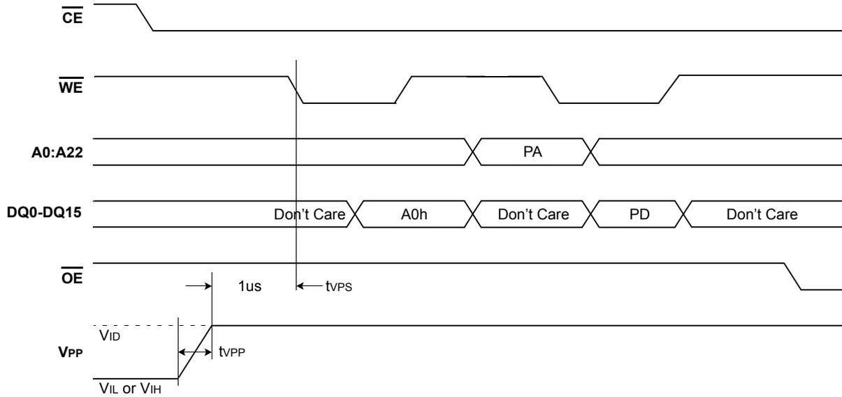
**Unlock Bypass Block Erase Operations**
