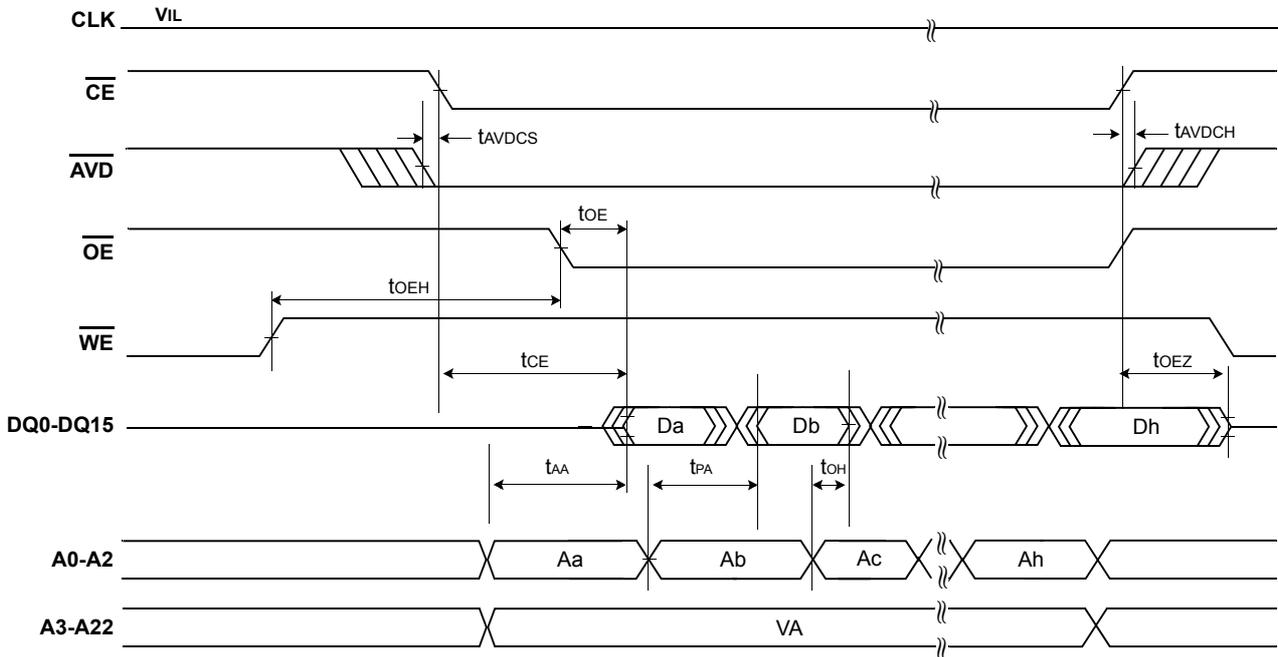
Figure 10: Asynchronous Page Mode Read
