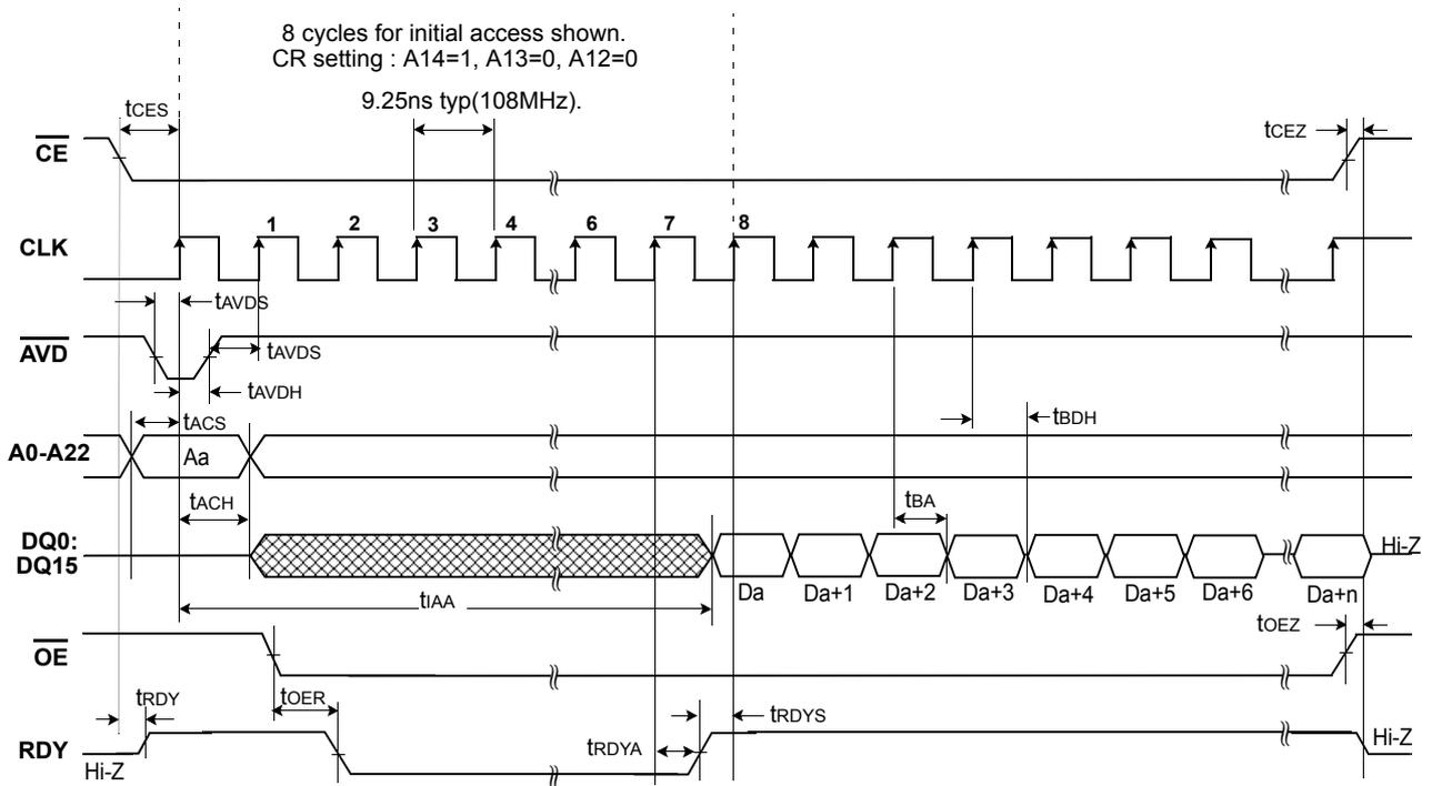
Figure 5: Continuous Burst Mode Read (108 MHz)
