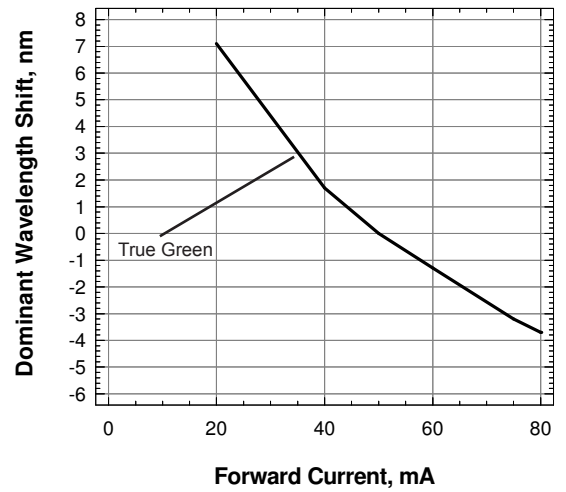
Dominant Wavelength Shift Vs Forward Current
