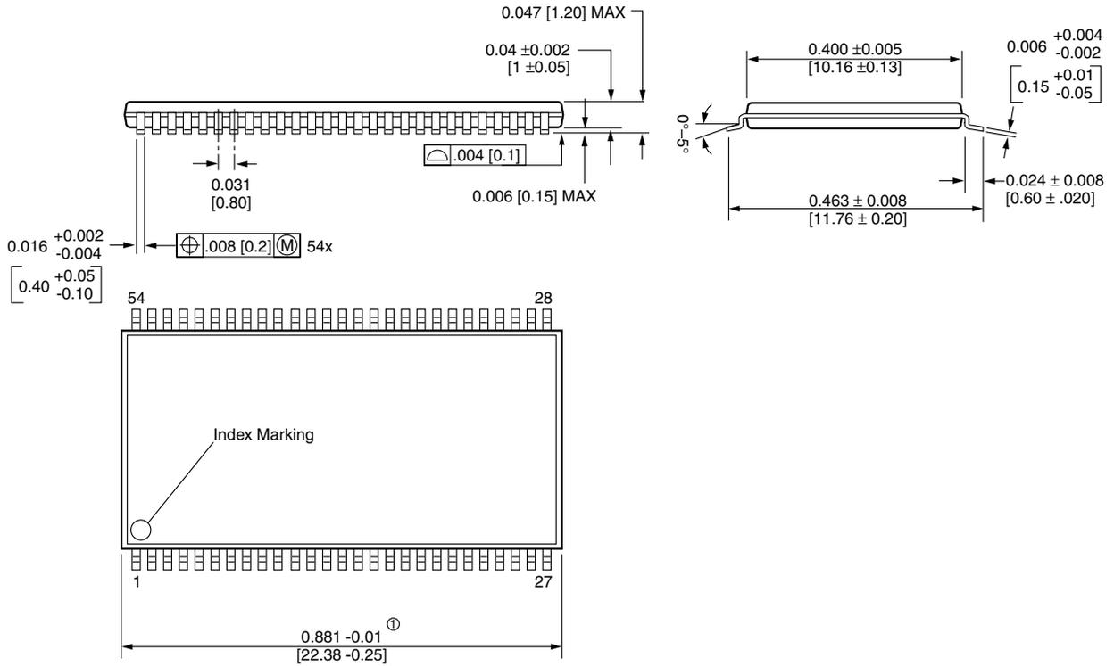
① Does not include plastic or metal protrusion of 0.15 max. per side
