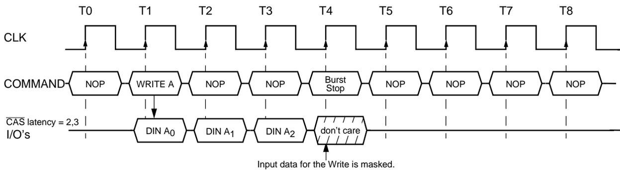
**9.1 AC Parameters for Write Timing**
