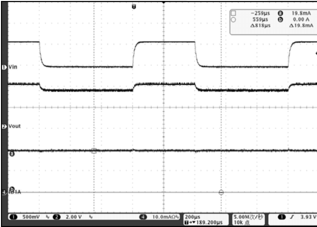
Figure 12. Line Transient Response in 1x Mode, V_{IN}=3.6V - 4.2V , I_{LEDx}=20mA
