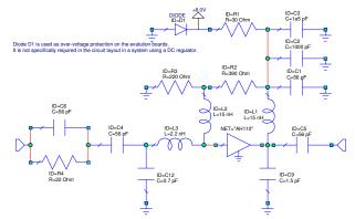
C12 is placed at silkscreen marker '1" or center of component placed at 43 deg. @ 1.9 GHz away from pin 1. C9 placed at silkscreen marker '8" or center of component placed at 39 deg. @ 1.9 GHz away from pin 3.
