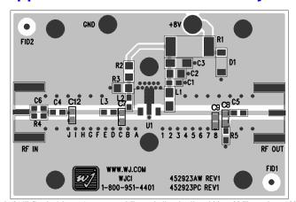
Circuit Board Material: .014" Getek, 4-layer, 1 oz copper, Microstrip line details: width = .026", spacing = .026"
