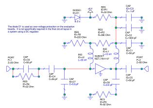
C7 is placed at silkscreen marker 'C' or center of component placed at 5.6 deg @ 900 MHz away from pin 1. C8 is placed at 22 deg. @ 900 MHz away from pin 3.
