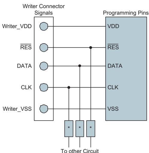
Note: \* may be resistor or capacitor. The resistance of \* must be greater than 1k $\Omega$  or the capacitance of \* must be less than 1nF.
