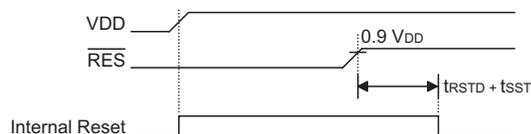
Note:  $t_{RSTD}$  is power-on delay, typical time=100ms
