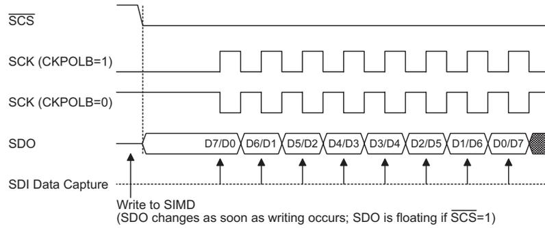
Note: For SPI slave mode, if SIMEN=1 and CSEN=0, SPI is always enabled and ignores the  $\overline{SCS}$  level.
