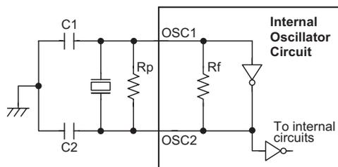
Note: 1. Rp is normally not required. C1 and C2 are required.
