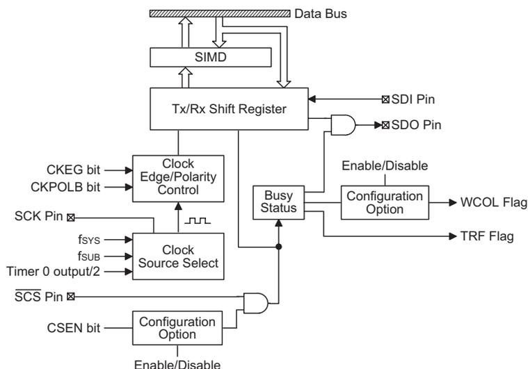
The status of the SPI interface pins is determined by a number of factors such as whether the device is in the master or slave mode and upon the condition of certain control bits such as CSEN and SIMEN.
