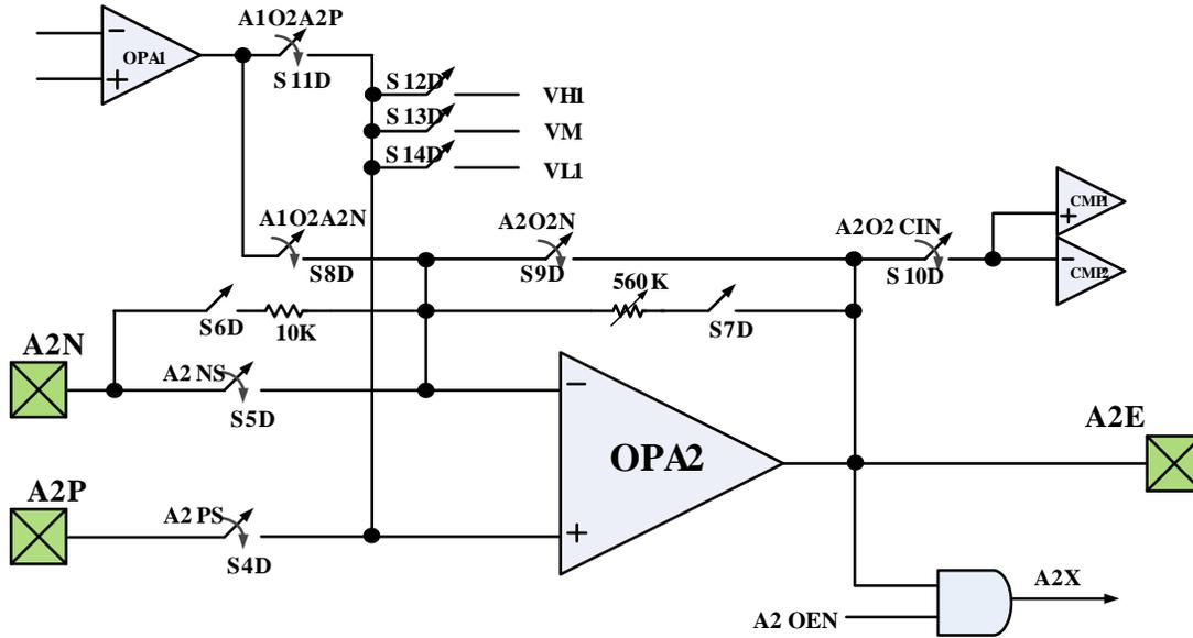
Switch priority S4D > S11D > (S12D, S13D, S14D); If A2PS=1, S11D~S14D will be opened by hardware.
