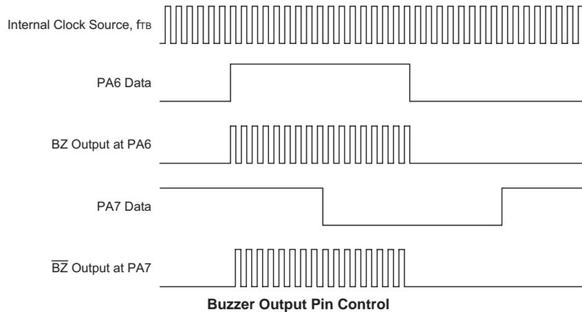
Note: The above drawing shows the situation where both pins PA6 and PA7 are selected by BPCTL option to be BZ and  $\overline{BZ}$  buzzer pin outputs. The Port Control Register of both pins must have already been setup as output. The data setup on pin PA7 has no effect on the buzzer outputs.
