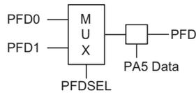
Note: 1. The PFD clock source, PFD0 or PFD1, which is from Timer0 or Timer1, is selected by PFDSEL bit in MISC register.
