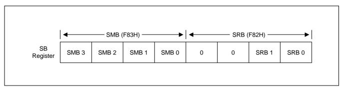
Figure 3-2. SMB and SRB Values in the SB Register
